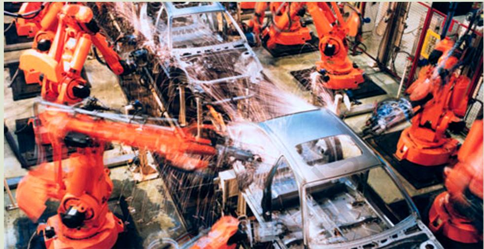
Figure 14.6 : Robot welding the car body
