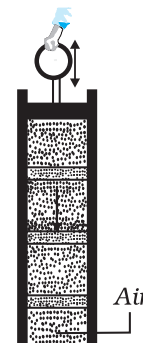
Fig. 14.4 Longitudinal waves (sound) generated in a pipe filled with air by moving the piston up and down. A volume element of air oscillates in the direction parallel to the direction of wave propagation.
