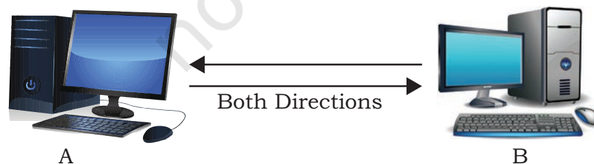
Figure 11.5: Full duplex transmission of data
