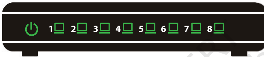
Figure 10.11: A network hub with 8 ports
