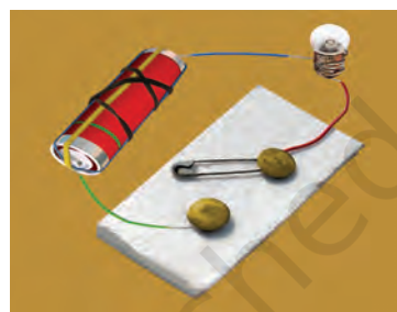
Fig. 9.9 An electric circuit with a switch
