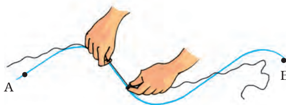
Fig. 7.10 Measuring the length of a curved line with a thread
