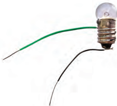
Fig. 9.4 Bulb connected to two wires
