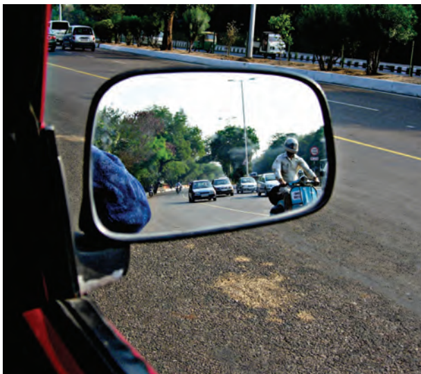
Fig. 11.20 Convex mirror as side view mirror
