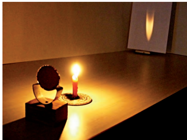
Fig. 11.15 Real images formed by a concave mirror
