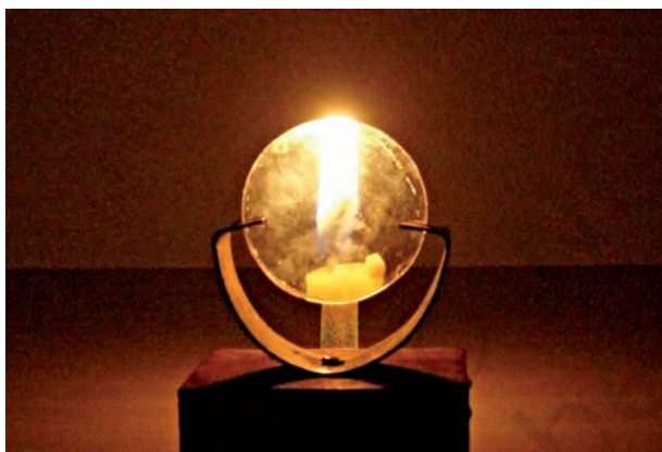
Fig. 11.26 Virtual image formed by the convex lens
