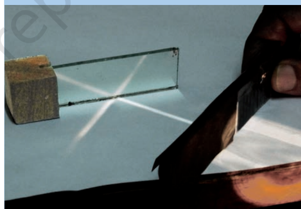
Fig. 13.1 : Arrangement for showing reflection
