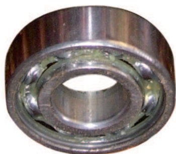
Fig. 9.16 : Ball bearings reduce friction
